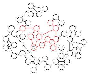
A *t*-round algorithm for the LOCAL model is a mapping from *t*-radius balls to valid outputs.
